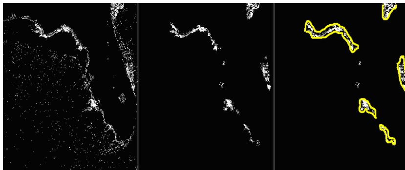
**Figure 1** Original image (left), after Spatial Density Filter (middle) and after the shape grouping (right)
